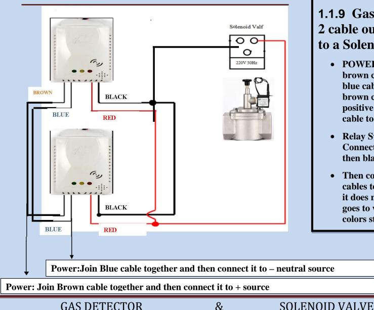
1.1.9 Gas Detector's with2 cable output installationto a Solenoid Valve:
